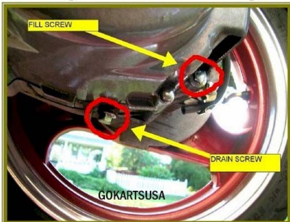
**Drain the Gear Oil.** Locate the Drain Screw at the bottom of the Final Drive
