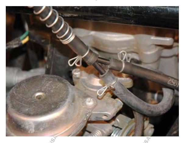
NOTE: Sometimes, the factory will plug the Y-connector into the Carburetor drain hose for shipment. If this is the case, disconnect the Y-connector, and then insert the Y-connector into the fuel tank's vacuum line.
