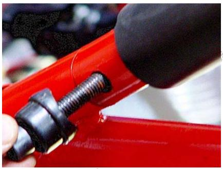
Once all bolts are inserted and well started, you can tighten all the bolts, starting from the bottom and working your way upwards
