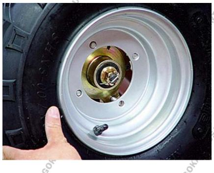
Install the lug nuts. The flat washer goes on first, then the lock washer, then the lug nut
