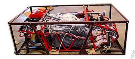
Remove all of the bottom bolts from around the crate and lift the upper part of the crate frame as one piece.
