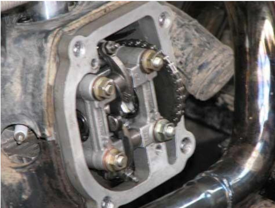
2. Rotate the camshaft until the big hole in the sprocket end points straight out of the top of the engine and the two smaller holes are lined up with the flat plane of the cylinder head. (Your camshaft may have lines instead of smaller holes, but they need to line up the same way). You can do this by rotating the variator in the CVT transmission counter clockwise by hand until the holes line up properly.
