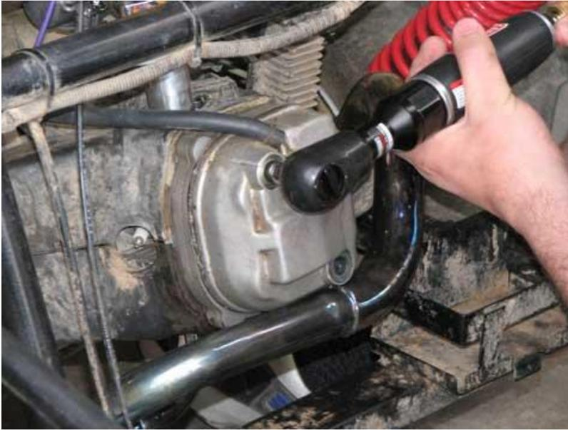
1. On some engine (kinroad) you may be able to adjust the valves directly on the engine. If not, remove the bolts holding the valve cover to the top of the engine.
