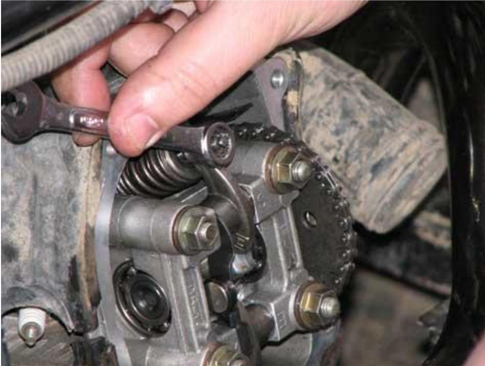
3. Use a wrench to loose the retainer nut on the intake (top) valve.
