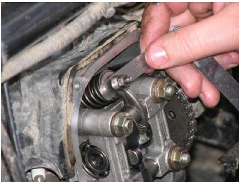
4. Using a feeler gauge, measure the gap between the top of the valve and the tappet of the rocker arm. Turn the tappet in or out as necessary to adjust. You want to set your valve clearances to 0.004" - 0.005" on both the intake and exhaust valves.
