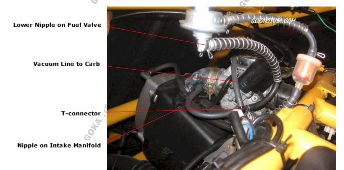
Connect the middle vacuum line on the T-connector to the top of the carburetor. Connect the left vacuum line on the T-connector to the nipple on the carburetor Intake Manifold
