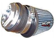
Place the clamp on the filter base. Slip the filter over the adapter. Tighten the clamp moderately to finger tight. Install Red Pre-filter (optional)
