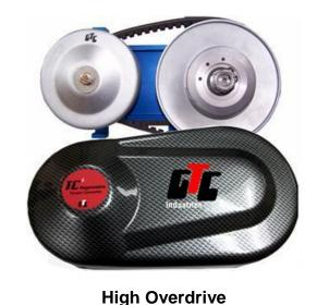
At maximum RPM, the Driven Pulley becomes fully open allowing the smallest possible diameter. At the same time, the Driver Pulley flanges are fully closed forcing the belt to its maximum diameter. This is High Gear Overdrive position
