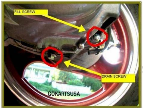
**Drain the Gear Oil.** Locate the Drain Screw at the bottom of the Final Drive
